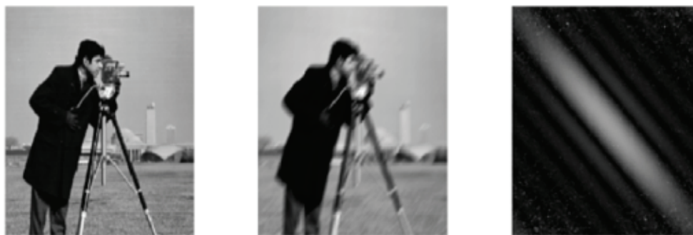
Fig. 2. Left: Sample image. Center: simulated camera motion at 45°. Right: Fourier transform of the center image
