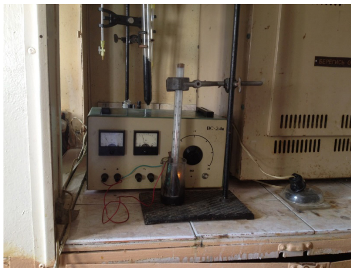
Fig. 2. Oxidation of pre-treated coal or graphite to produce mellitic acid
