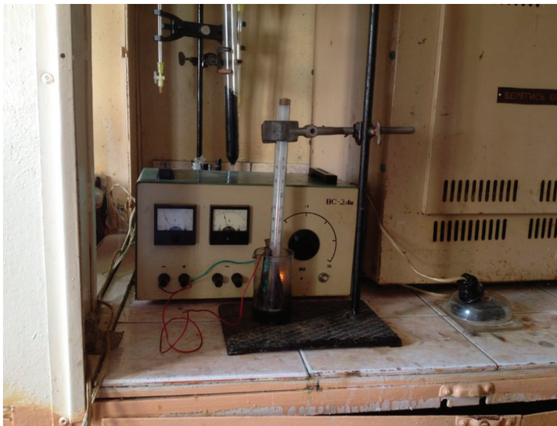
Fig. 2. Electrochemical process of pre-treated coal or graphite to produce mellitic acid
