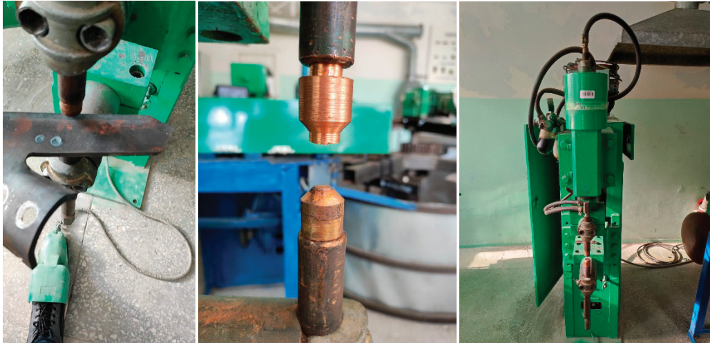
Fig. 4. Installation for spot welding MT-1222
