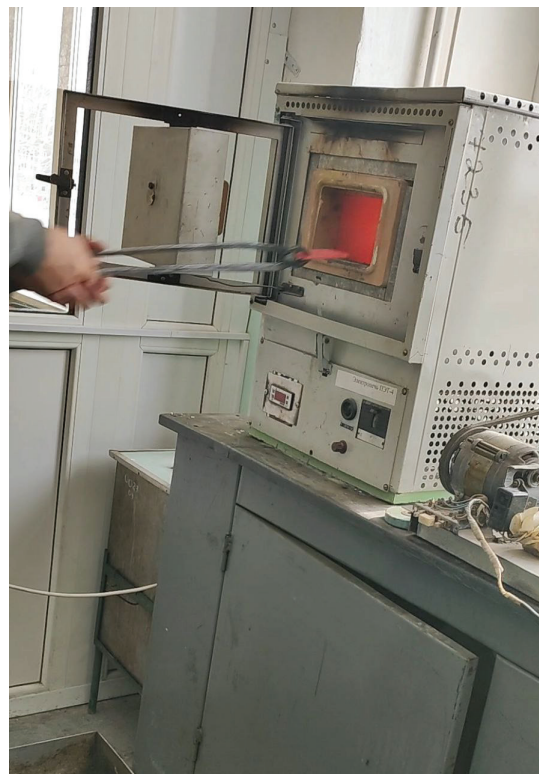
Fig. 6. Muffle furnace PET-4
