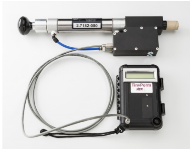
Fig. 1. TinyPerm for permeability measurements, New England Research, http://www.ner.com/
